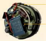
Integrated electronic and power supply board
